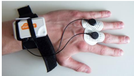
Figure 2: The Shimmer2r GSR sensor measures the skin conductance between two electrodes attached to e.g. the finger or the forearm.
