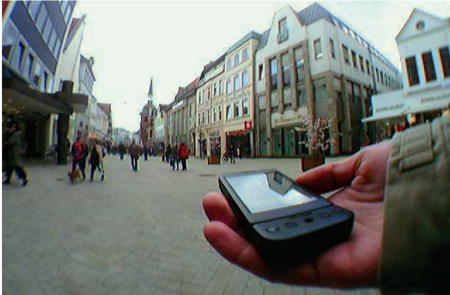
Figure 3.9: Scanning is a novel interaction technique and often used in the domain of pedestrian orientation and navigation systems. A user holds a mobile phone almost parallel to the ground, points it to varying directions, and receives feedback.
