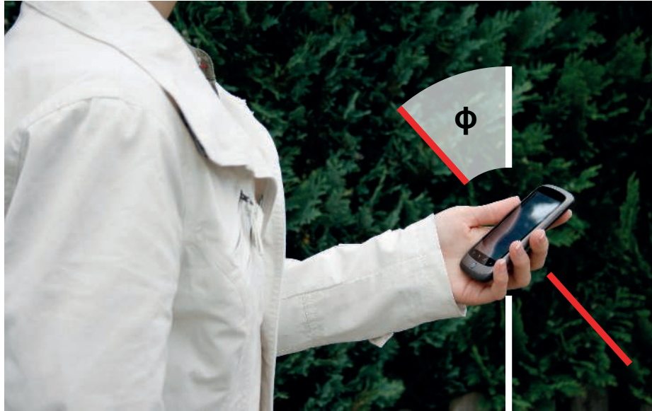
Figure 3.10: A scan event was defined if roll and pitch angles both are between -16^\circ and 16^\circ . This visualisation shows how the pitch angle is defined.
