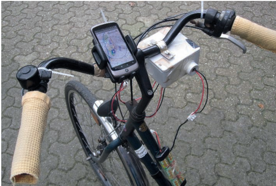
Figure 6.2: The Tacticycle consists of two core components: a mobile phone, which serves as visual display, and two vibration actuators in the handlebars. Both components are connected via custom-made hardware.
