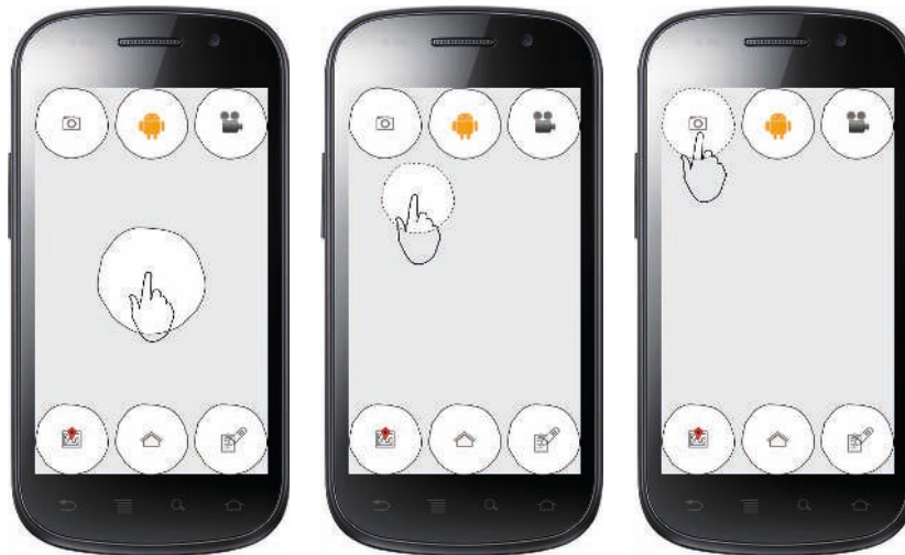
(a) Step 1: Select centred icon. (b) Step 2: Drag bubble towards desired functionality. (c) Step 3: Release when finger is above desired functionality.
