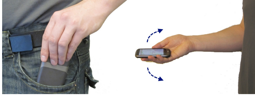
Fig. 3. The PocketNavigator offers two modes: the pocket mode (left) and the scanning mode (right). If the scanning mode is activated, the device uses the compass to detect the pointing direction and the bearing to the next waypoint. If the device is in the pocket, the GPS heading is used instead.
