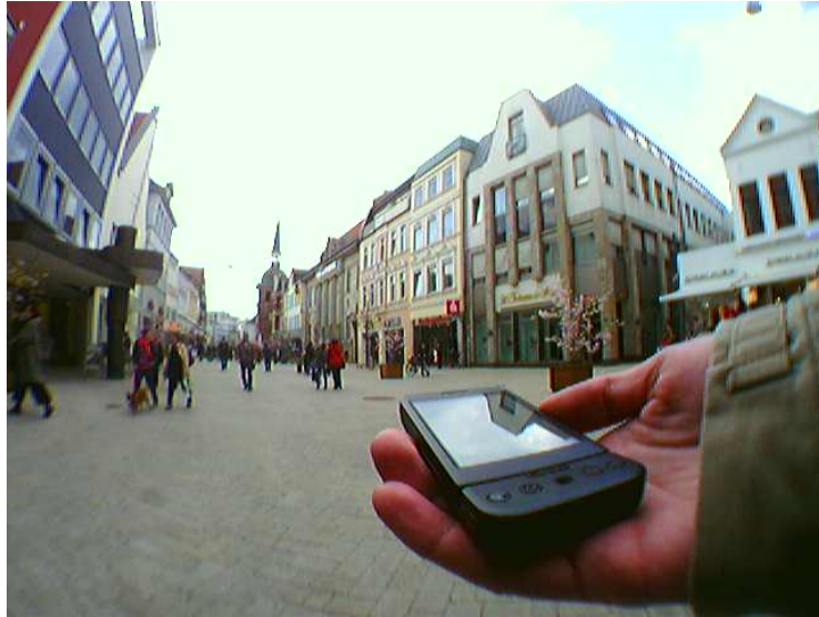
Fig. 1. Scanning is a novel interaction technique and often used in the domain of pedestrian orientation and navigation systems. A user holds a mobile phone almost parallel to the ground, points it to varying directions, and receives feedback.
